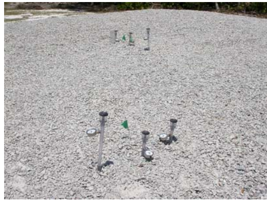
F. Close-up of tensiometer arrays.
