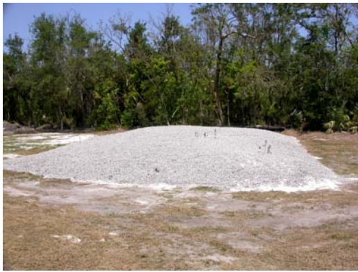
E. Granite mulch (3") and tensiometers.
