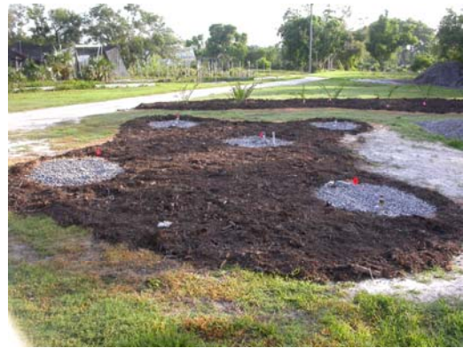
J. Five of the pits with tensiometers.
